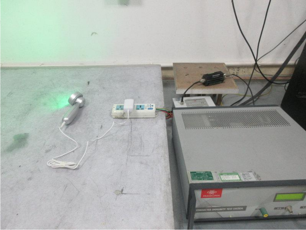
Photo of Injected currents susceptibility Test
