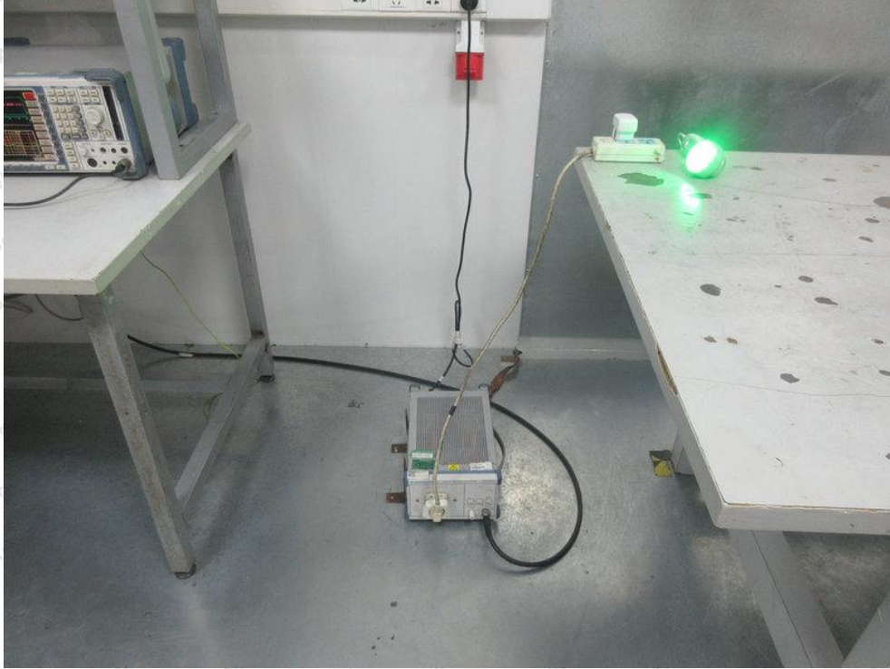
Photo of Power Line Conducted Emission Test
